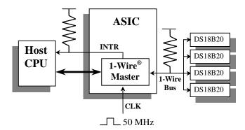
Figure 1 shows the circuit configuration this example will refer to. The 1-Wire Master has been designed into a customer ASIC and the host CPU will use it to order four thermal sensors to convert temperature and report their values. The 1-Wire bus and the INTR line each have a standard 5k pull-up resistor attached. A 50 MHz system clock drives the 1-Wire Master's timing through the CLK pin. The 1-Wire Master has been memory mapped into port address space of the CPU.
